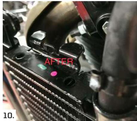
Install the scoop over radiator top tabs & slide lower mount tabs between the frame rails until the mount holes in scoop align with the holes in the frame. Install the (2) 3/8 - 16 x 1" hex bolts w/ flat & lock washers. Loosely snug. Check upper tab fitment for a snug fit & gently bend tabs to snug up if needed. (Fig #11 - 13)
