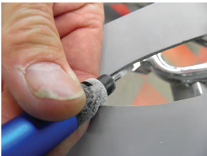
07. Bevel the edge back so you can't see the thick wall of the fender or bag through the lens once installed.
