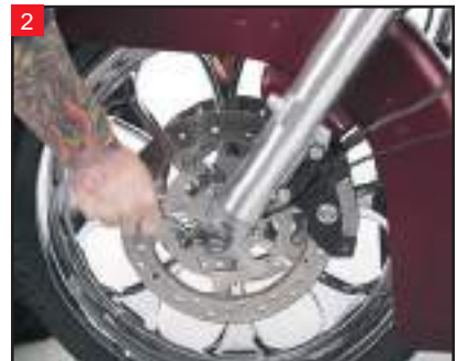
2 Loosen the front axle nut, but do not remove it at this time.
