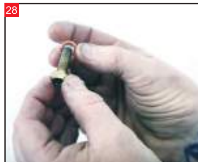
Use a NEW crush washer on the damper tube bolt.
