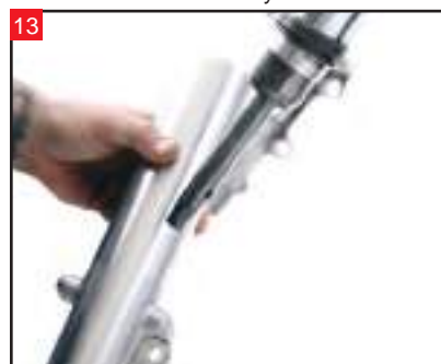
Remove the lower fork slider from the fork leg, exposing the damper tube.
