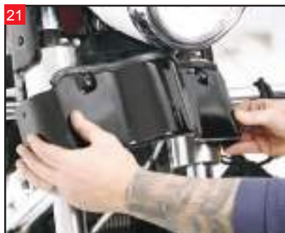
With the two bolts removed, you can remove the outer fairing. There may be a wiring connector attached if the bike is ABS equipped.
