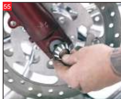
Install the right side axle cap and bolt. Use the 1" bolt for this side.
