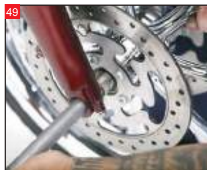
49 Start the "Yaxle" from the right side of the motorcycle, installing the left side spacer when you get through the wheel hub.
