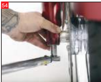
Torque these bolts to 15-18 foot/lbs.
