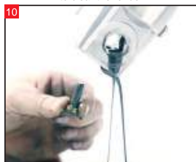
With the long 6mm Allen, and impact wrench, remove the damper tube bolt from the bottom of the fork leg. Have your drip pan ready, as the fork oil will come out when you remove the bolt.
