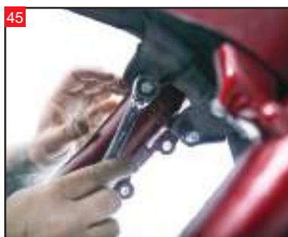
45 Using a 1/2" wrench, tighten the front fender bolts to 16-20 foot/lbs.
