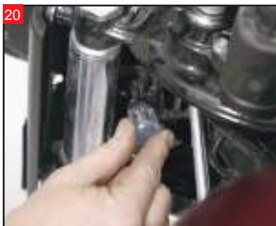
Use a Torx bit to remove the bolts that retain the lower outer fairing.
