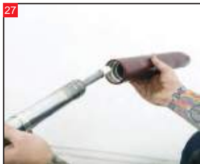
With the damper cup in place on the tube, install the fork leg into the lower fork slider.
