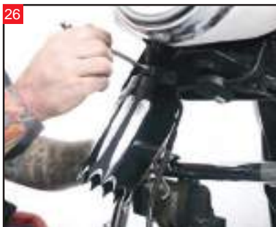
Apply removable thread locker (blue), to the bolts you just removed, and use them to install the new "Yafterburner" upper fork slider covers. Tighten these bolts to 90-120 inch/lbs.
