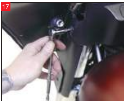
Use a Torx bit to remove the bolts holding the lower inner fairing.
