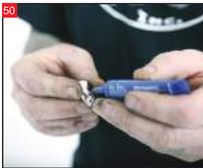
50 Apply a small amount of thread locker (red) onto the bolts that come with the "Yaxle".
