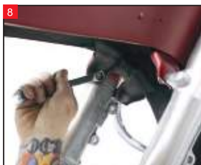
Using the 1/2" wrench, remove the fender mounting bolts.
