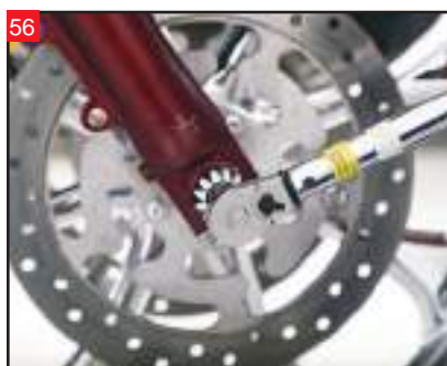
Torque the right side to 20 foot/lbs.
