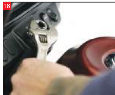
Using an adjustable or 7/8" open-ended wrench, remove the locking nut on the ignition switch post. All parts will lift up and off with the nut removed.
