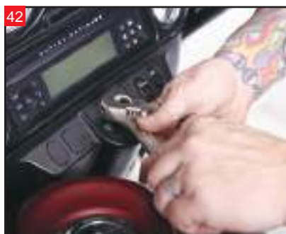
42 Re-install the components onto the ignition switch post, and tighten the lock nut.
