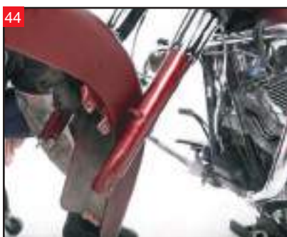
44 Position the front fender in place, and start the four bolts.
