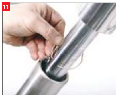
Gently bring the fork slider down, to access the retaining ring above the seal. Using a small flat-tip screwdriver, remove the ring.
