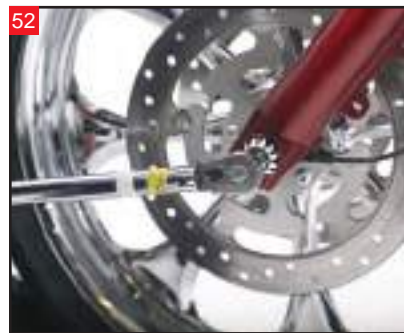
52 Torque the left side bolt to 30 foot/lbs.
