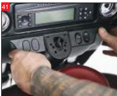
41 The inner lower fairing/ignition switch cover goes on next. Don't forget to plug in the switch wiring.
