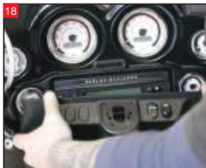
Remove the lower inner fairing. Do not pull it out too far, there are wires to disconnect.
