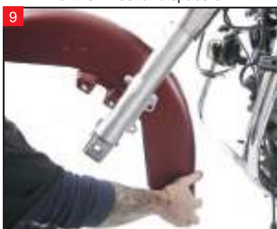
Remove the front fender.
