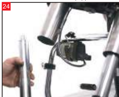
Slide the fork leg out and free from the triple trees.
