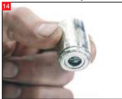
Check inside the fork slider, as the damper tube cup often stays inside. You will need this cup for reassembly.
