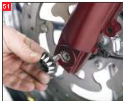
51 Install the left side bolt first, with the end cap. Use the 1.5" bolt.
