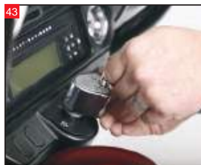
43 Install the ignition switch.
