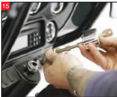
Remove the ignition switch. Do this by turning the key past the lock position, and compressing the detent on the bottom of the switch. Pull the switch straight up.
