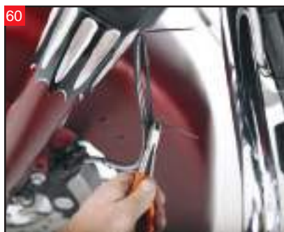
Trim the excess from the ties.
