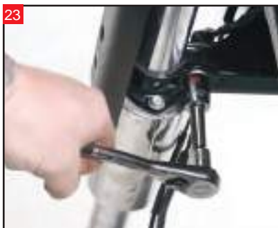
Maintain control of the fork leg, and use a 5/8" socket to remove the pinch bolt from the lower triple tree.
