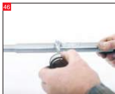
46 Apply a small amount of anti-seize to the new "Yaxle".
