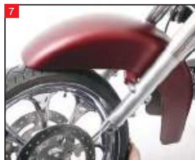
With the axle removed, remove the wheel from the front end. This may require you to raise the motorcycle in order to clear the fender.
