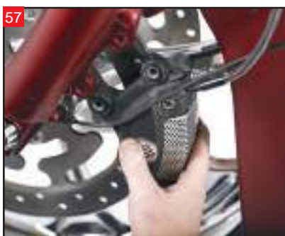
Re-install both front brake calipers.
