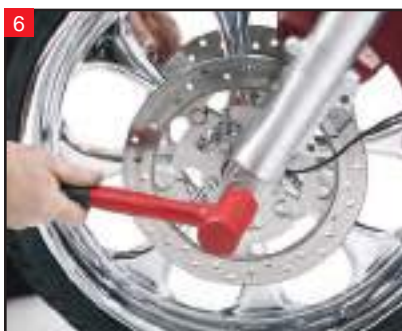
With the axle nut, washer, and lock washer removed, use a rubber mallet to gently tap out the axle. Maintain control of the wheel and spacers.
