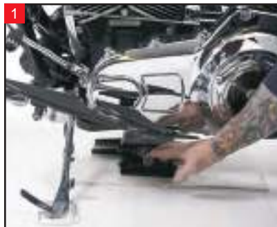
1 Start by using the floor jack to support the weight of the bike, getting the front end off the ground.
