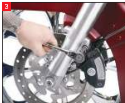
3 Using the 10mm, 12 point socket, remove the bolts holding the front brake calipers to the forks.
