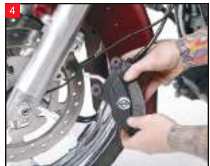
4 Cut the ties that hold the brake line to the ABS sensor wire, (if equipped), remove the caliper.
