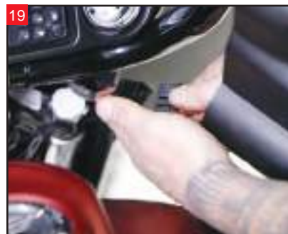
Disconnect the switch wiring once you have access to it.
