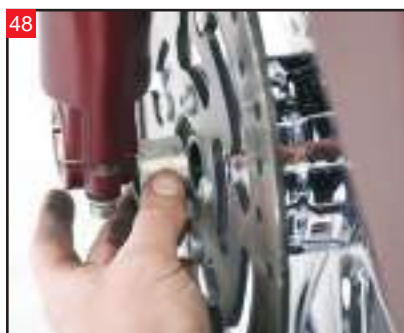
48 Place the right side wheel spacer in position, between the wheel and fork.
