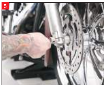
Loosen the right side fork clamp using a 1/2" wrench or socket.
