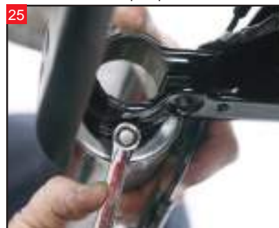
Using a 3/8" wrench or socket, remove the two bolts that hold the upper fork slider covers from the lower triple tree.
