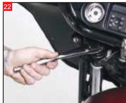
With the lower fairing components removed, you can now remove the fork legs. Start by loosening the top cap bolt.
