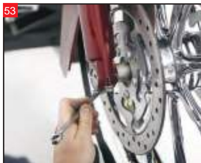
Tighten the right end cap nuts evenly.
