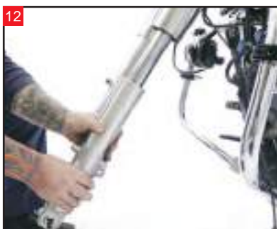
Next use a "slide-hammer" motion to free the fork seal.
