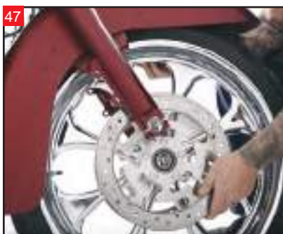
47 Position the front wheel back in it's position.
