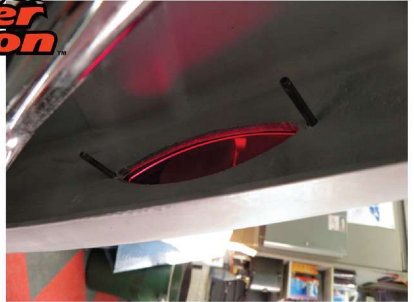
10. Slide the bezel with the set screws installed through the fender / bag and then slide the light box over the two studs and secure it with the two nuts provided.
