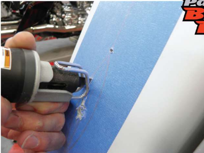
5. Using a reciprocating saw cut along the inside of the inner bezel area that you marked.
