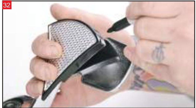
Holding the Wedgy Super Bling pedal in place, mark the location to cut the stock brake pedal with a permanent marker.
