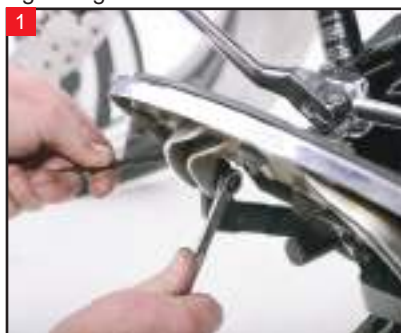
With a 3/16" Allen and 7/16" wrench, remove the floorboard mounting hardware.
