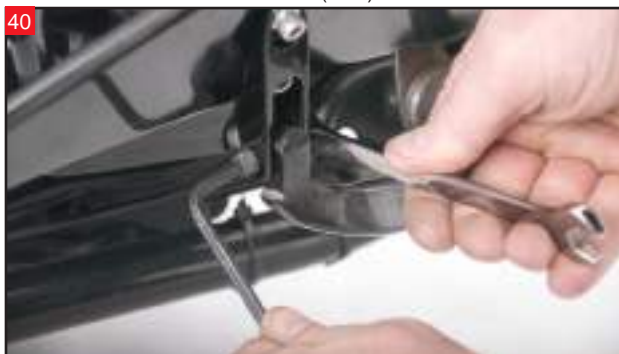
Fasten the Wedgy Floorboard to the mounting brackets using the stock hardware.
