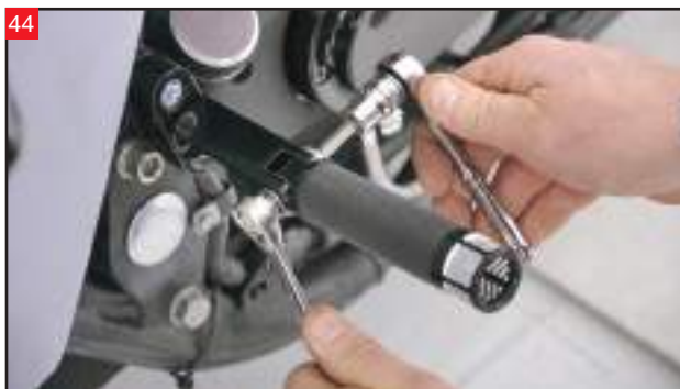
Use the second 3/8" bolt, washer, and nylock nut to hold the passenger peg to the mount.
