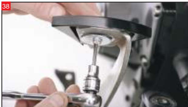
Remove the bike cover from the motorcycle. Install the Wedgy Brake Pedal with the included hardware. Use thread locker (blue) on the bolt.
