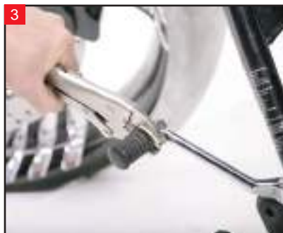
A set of vice grip pliers makes removing the stock rubber shift peg easier.
