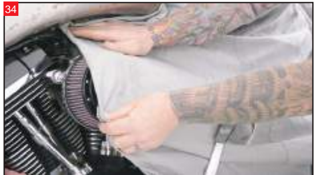
Use an old bike cover or sheets to protect the rest of the motorcycle from sparks and debris.
