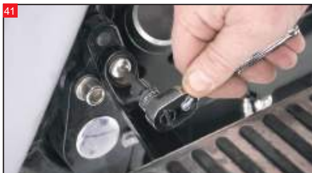
Use an Allen wrench to remove the right side passenger floorboard and mounting bracket.
