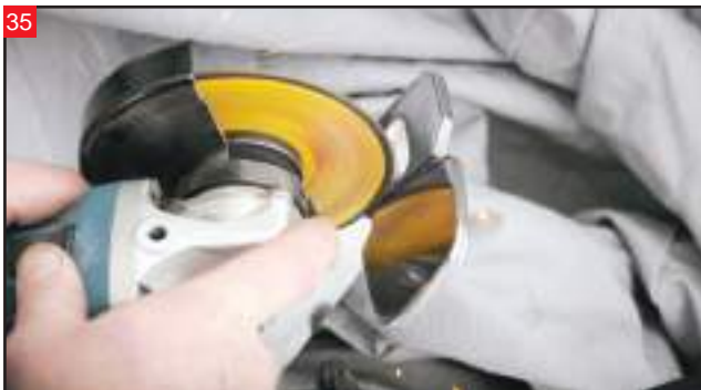
Using the angle grinder with cut off wheel, cut the pedestal of the stock brake pedal on the line you made. IMPORTANT: Wear eye protection during this step.
