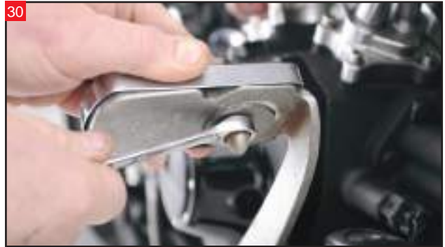
With a 1/2" wrench, remove the acorn nut holding the cover to the stock brake pedal.
