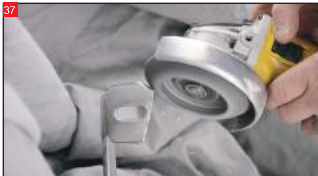
Use a sanding disc to clean up any rough edges from your cut. IMPORTANT: Wear eye protection during this step.
