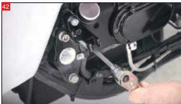
Install the Drag Specialties/Hotop Passenger Peg Mounting Bracket to the frame as done on the left side.
