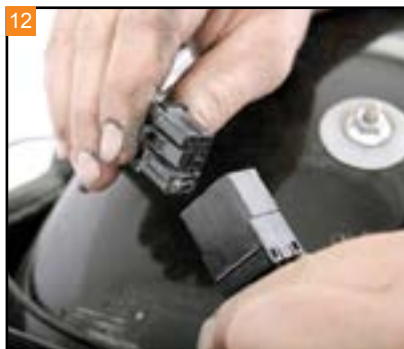
12 Unplug the rear wiring harness at the front of the rear fender.
