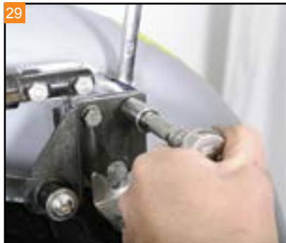
29 Final tighten all fender mounting hardware, including the hardware for the license plate eliminator. Be sure to use thread locker on all hardware.
