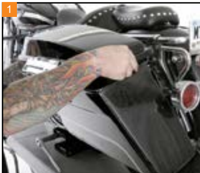
1 Remove both saddlebags and seat. Disconnect the negative terminal of the battery.
