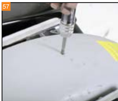
Create threads in the hole with a 1/4"x20 tap.
