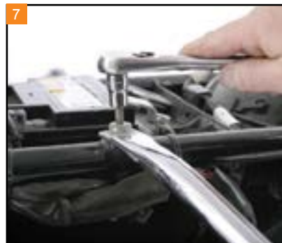
7 Use a T40 Torx to remove the hardware at the front of the saddlebag support bracket. The lower bolt requires a 9/16" wrench.
