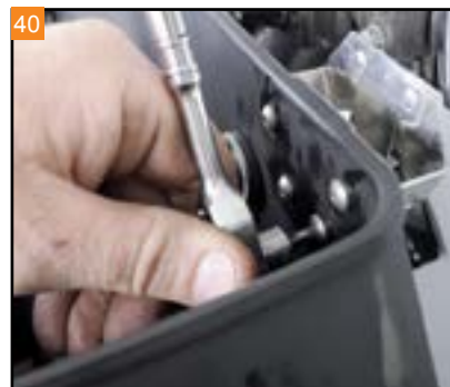
40 With a T40 Torx, use the stock hardware to install the mounting brackets on the new saddlebags.
