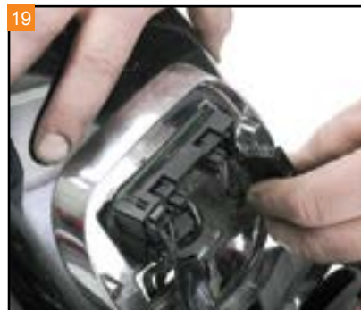
19 With a Phillips screwdriver, remove the two screws holding the taillight lens to the fender. Unplug the harness from the taillight circuit board inside.
