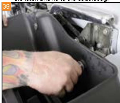
39 Use the bail pins to secure the saddlebags to the brackets. Start with the rear bail pin first. After the front bail pin is installed, tighten the bolt for the bracket.
