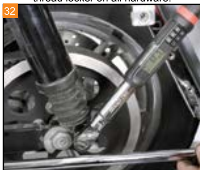
32 Lower the frame with the center jack. Reinstall the lower shock mounting bolts. Using blue thread locker, final torque to 35-40 foot/lbs.
