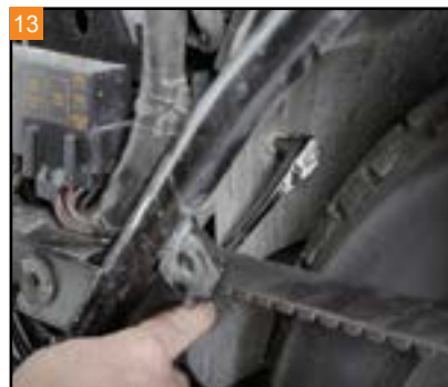
13 Raise the frame of the motorcycle, with the rear wheel on the lift to access the bolt at the front of the rear fender. Remove the bolt with a T40 Torx.
