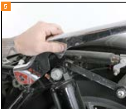
5 Lift the chrome cover off the fender strut of the frame.
