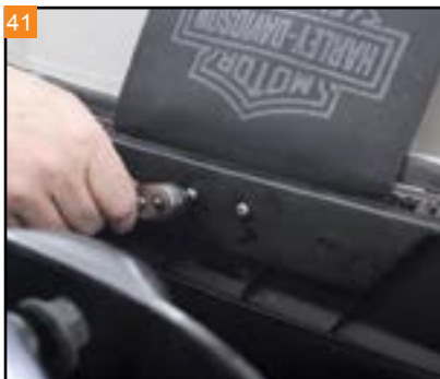
41 Bring the lid into position. Start all four bolts that mount the latch to the saddlebag. Final tighten the two inside bolts, then remove the two outer bolts in order to attach the tether strap.
