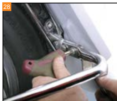
28 Use a T40 Torx and 1/2" wrench to tighten the bolts at the rear of the saddlebag support.
