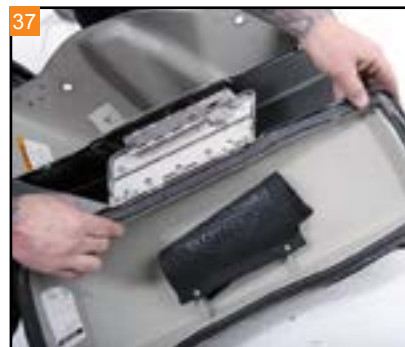
37 Remove the lid from the saddlebag. Repeat the process for the second saddlebag.
