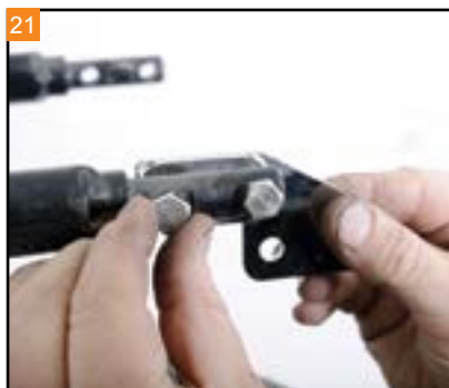
21 Using the stock bolts and hardware that came in the kit, install the brackets from the license plate bar eliminator kit. Leave the bolts loose for now.
