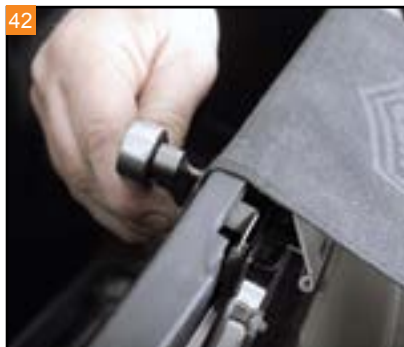
42 Bring the tether strap into position. Reinstall the two outer bolts with a T15 Torx.
