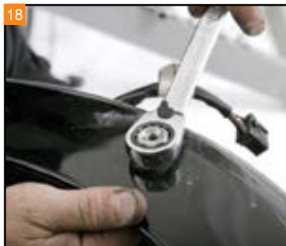
18 Use a 3/4" wrench to remove the fender mounting hardware from the stock fender.
