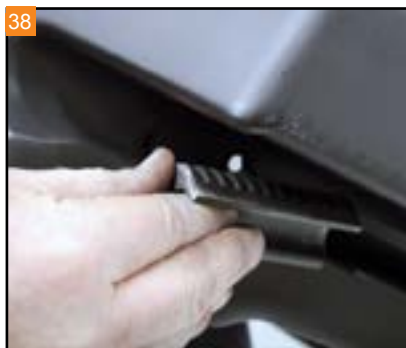
38 Install the cushions into the channel of the Drag Specialties Extended Saddlebags. A small amount of lubricant will help seating the tip in the hole. Also install the bail pin grommets.
