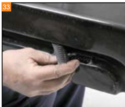
33 Remove the saddlebag support cushions from the channel at the bottom of the stock saddlebags.
