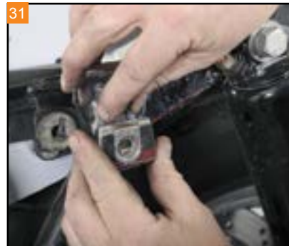
31 Start the front saddlebag bail pin brackets, leaving the bolt loose for now.
