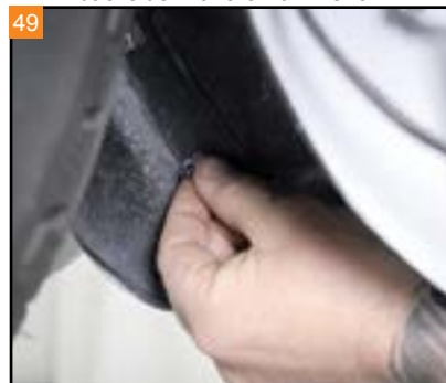
49 Install the hardware for the license plate frame from the inside of the fender.
