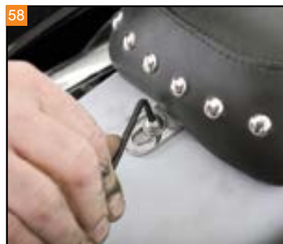
Reinstall the seat on the motorcycle. Secure the seat with a 1/4" seat bolt.
