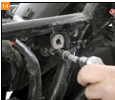
14 The last two fender bolts to be removed are located near the rear most side cover gromets. Use a T40 Torx to remove. Maintain control of the fender while doing so.
