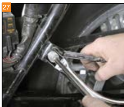
27 With all the hardware installed, tighten the bolts at the front of the saddlebag support bracket.
