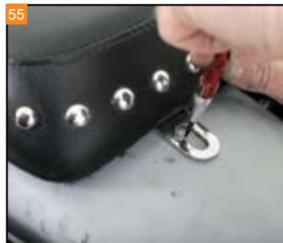
Mark the location of the hole for the seat bolt with a center punch.
