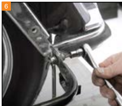
6 With a T40 Torx and 1/2" wrench, remove the hardware holding the saddlebag support bracket to the rear fender bracket.
