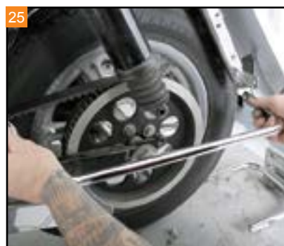
25 Position the Drag Specialties' Saddlebag support brackets. Start the front bolt and nut with a T40 Torx and a 9/16" wrench.
