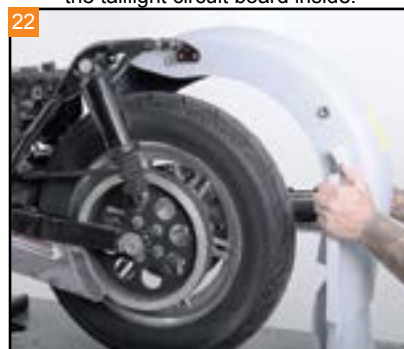
22 Bring the Bagger Nation fender into position between the fender struts of the frame.
