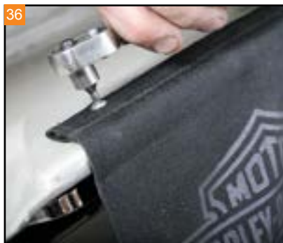
36 Remove the two screws holding the tether strap to the latch. With the tether removed, loosen the two remaining bolts holding the latch and lid to the saddlebag.
