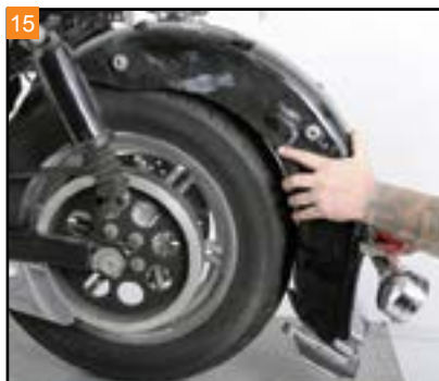
15 Remove the rear fender from the motorcycle.
