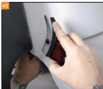
45 Position the left Wedgy Light into the pockets of the filler panels. The lights are left and right specific.
