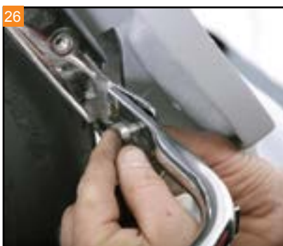
26 Install the four bolts and nuts that hold the rear fender bracket, saddlebag support brackets, and rear fender supports together.
