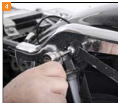
4 Use an Allen wrench to remove the docking point behind the rear shock.
