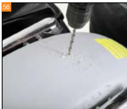
Remove the seat. Drill a hole at the mark with a 13/64" drill bit.
