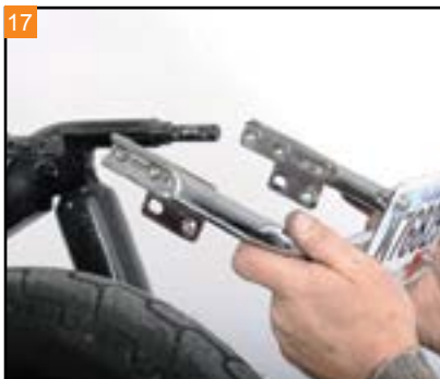
17 Remove the license plate bar by sliding it out from the rear of the motorcycle.
