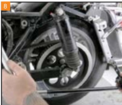
8 Remove the stock saddlebag supports from the motorcycle.
