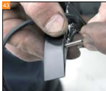
43 Start the included studs into the back of the Wedgy Light Housings.
