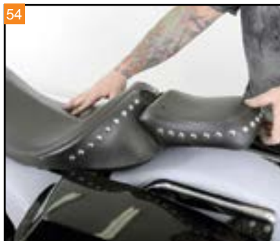
Bring the seat into position. Be sure the tab at the front of the seat engages in the slot in the frame.
