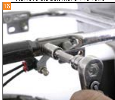
16 Use a 1/2" socket to remove the four bolts holding the license plate bar from the frame.
