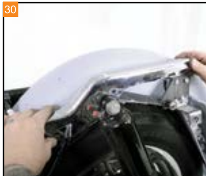
30 Reinstall the chrome covers over the fender struts of the frame. The piece may need to be trimmed to fit properly.
