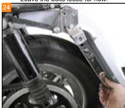
24 Reinstall the fender support brackets on each side of the rear fender. Leave the hardware loose.
