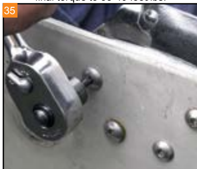
35 Use a T15 Torx to remove the eight screws per saddlebag holding the brackets.
