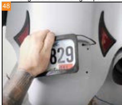
48 Remove the license plate from the stock bar. Trim to fit the Bagger Nation lighted license plate frame. Install the license plate and frame in the pocket of the fender. Feed the wires through the pre-drilled hole.
