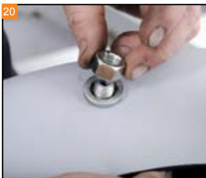
20 Install the fender mounting hardware onto the Chupa fender. The fender has pre-drilled square holes to accept the hardware.
