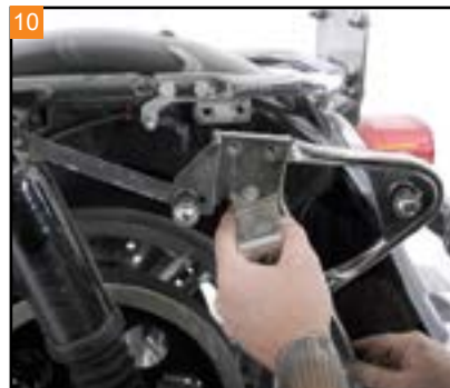
10 Remove both fender support brackets from the license plate bar.
