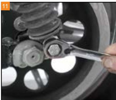
11 Support the motorcycle's frame with a center jack. With a 3/4" wrench, remove the lower shock mounting bolts.
