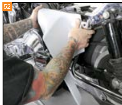
52 Ensure the wires are zip tied away from any moving parts. Install the Swoop Side Covers in the stock location.
