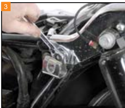
3 With a 7/16" wrench, loosen the hex bolt holding the front saddlebag bracket.
