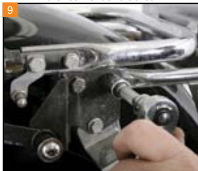
9 With a 1/2" socket, loosen the two bolts at the fender support brackets.
