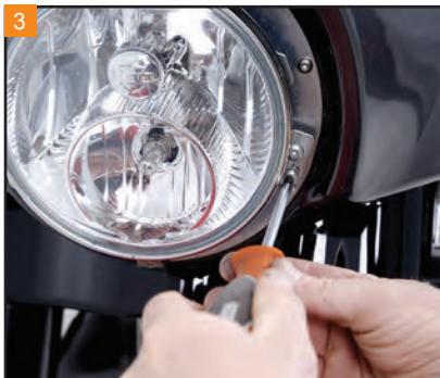
3 Use a Phillips screwdriver to remove the screws for the retaining ring of the headlight.
