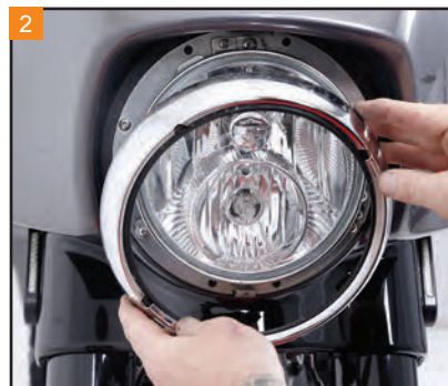
2 Rotate the trim ring counter-clockwise and remove from the headlight.
