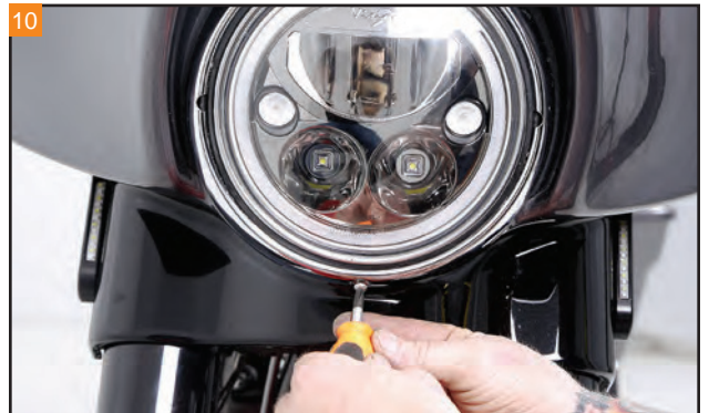
After positioning the trim ring, use a Phillips screwdriver to install the screw at the 6 o'clock position.
