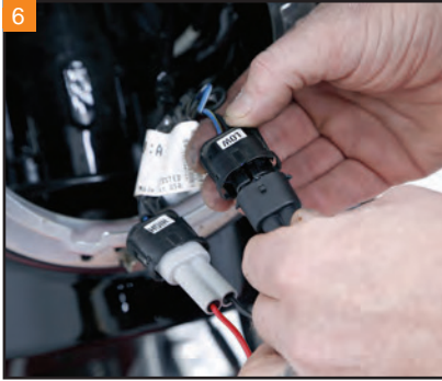
Plug the included adapter harness into the stock wiring.
