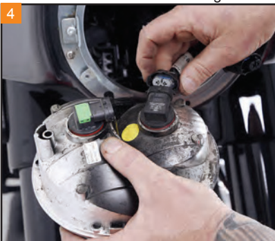
4 Remove the headlight from the fairing. When accessible, disconnect the wiring connectors from the back of the headlight.
