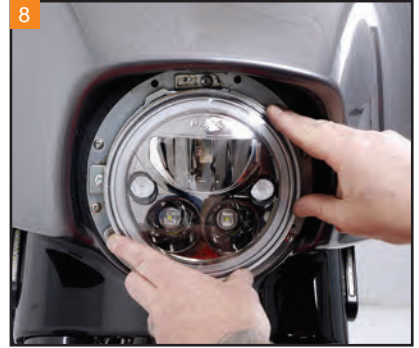
Position the Never Night Headlight in the stock location.
