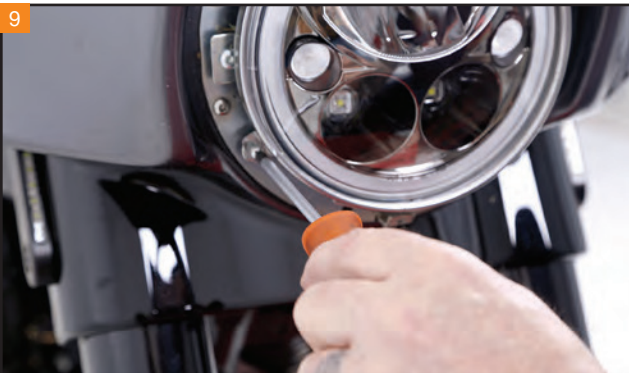
Reinstall the retaining ring with stock hardware.
