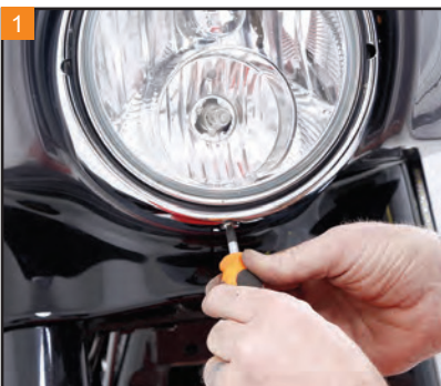
1 After installing a fender cover to prevent damage, use a Phillips screwdriver to remove the single screw at the bottom of the trim ring.
