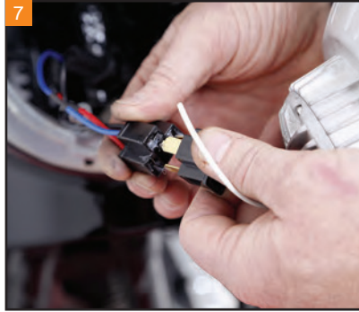
Plug the headlight into the single connector of the adapter harness.
