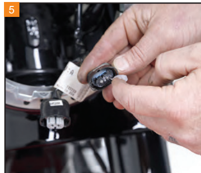
5 Apply a small amount of dielectric grease to the stock connectors, as well as the connectors on the Bagger Nation wiring adapter.
