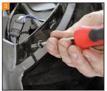
Temporarily reinstall one of the windshield screws to hold the outer fairing while the other hardware is removed.
