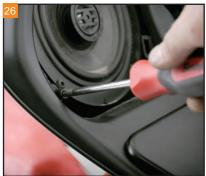
Tighten the bolt on each side of the speaker with a T30 Torx.
