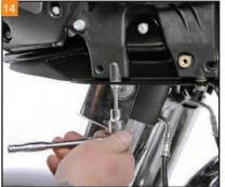
Tighten the lower bolt on each side with a 5/32" Allen. Go back and final tighten the upper stock bolt installed first.
