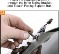
Use a windshield screw to hold the outer fairing while installing the remaining hardware.
