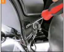
With a T27 Torx, remove the two remaining bolts holding the outer fairing.
