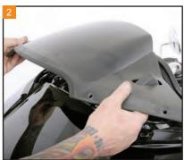
Lift the air vent assembly straight up and off the fairing.
