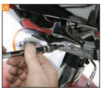
With a 3/16" Allen wrench, install the bolts behind the front turn signals.
