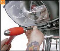
Use a center punch to mark the two holes to be drilled at the front of the inner fairing.
