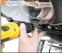
Drill two small pilot holes in the inner fairing support bracket.
