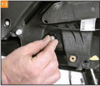
Hold the Stealth Fairing Support Bar in place by loosely installing the stock bolt.
