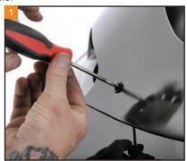
Use a Phillips screwdriver to remove the windshield hardware. Remove the windshield from the fairing.
