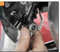
Use a T27 Torx to tighten the two bolts at the bottom of the inner fairing.
