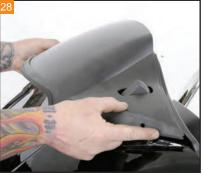
Bring the air vent assembly back into position.
