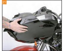
Slide the outer fairing back into position.
