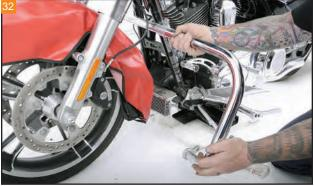
Slide the engine guard out from the side of the motorcycle.
