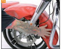
Place a fender cover over the front fender to protect the painted finish.
