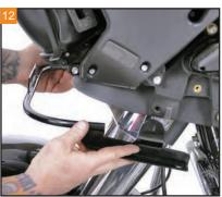
Bring the Bagger Nation Stealth Fairing Support Bar into position at the front of the inner fairing.
