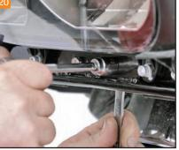
Use removable thread locker on the hardware. Tighten the hardware with a 1/2" wrench and socket.
