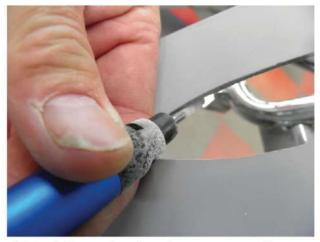
Bevel the edge back so you can't see the thick wall of the fender or bag through the lens once installed.
