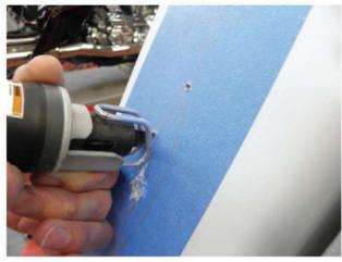
Using a reciprocating saw, cut along the inside of the inner bezel area that you marked.
