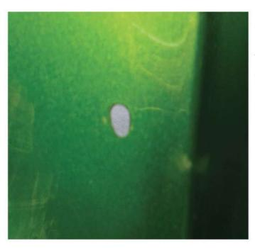
2. The templates are marked with hole sizes for drilling. We recommend drilling a small pilot hole first to avoid drill bit walk and then drilling the final hole size in a second operation. Also now is a good time to OBLONG the top and bottom 3/16 hole that you have just drilled this will allow for easier install further into the process.
