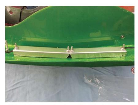
Note: When snugging down the nuts, hold onto the studs (set screws) with an Allen wrench to prevent the studs from over-tightening into the bezel.
