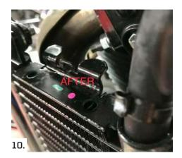
Install the scoop over radiator top tabs & slide lower mount tabs between the frame rails until the mount holes in scoop align with the holes in the frame. Install the (2)  $3/8 - 16 \times 1$ " hex bolts w/ flat & lock washers. Loosely snug. Check upper tab fitment for a snug fit & gently bend tabs to snug up if needed. (Fig #11 - 13)
