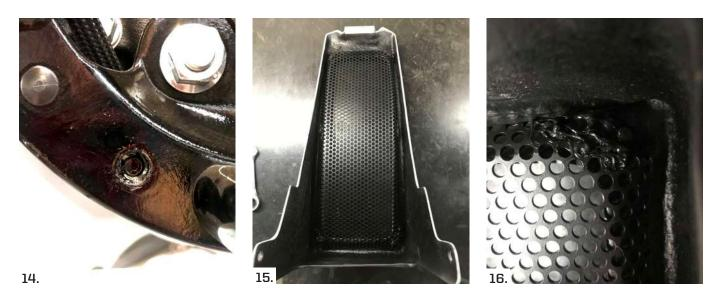
5. Remove Chin Scoop & paint... Silicon or epoxy grill inside...final install (Fig #15 - #18)
