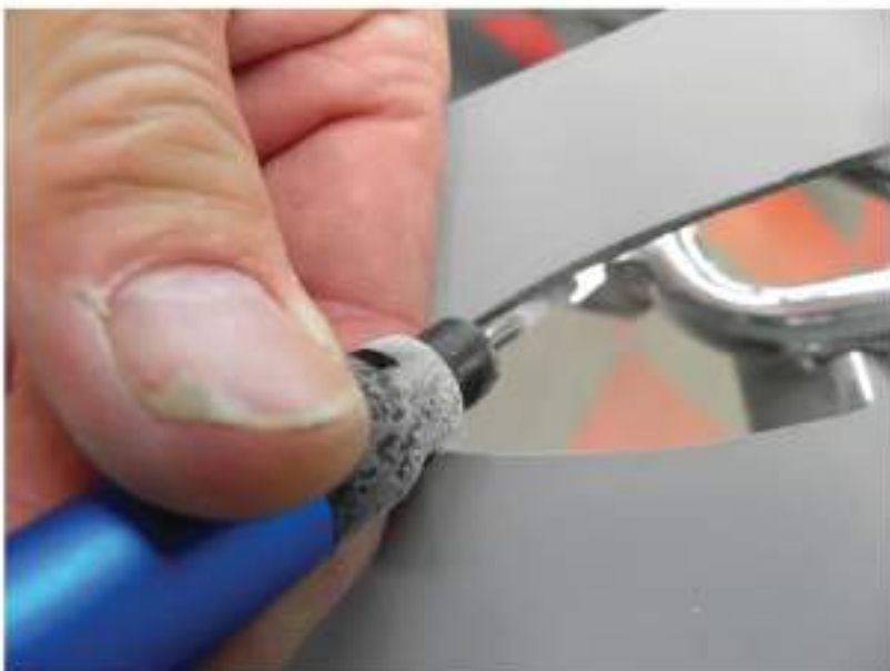
7. Bevel the edge back so you can't see the thick wall of the fender or bag through the lens once installed.
