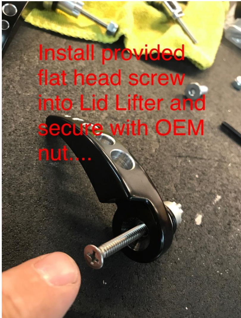
5. Install provided flat head screw into Lid Lifter and secure using OEM nut
