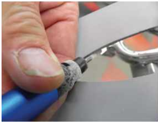
7. Bevel the edge back so you can't see the thick wall of the fender or bag through the lens once installed.
