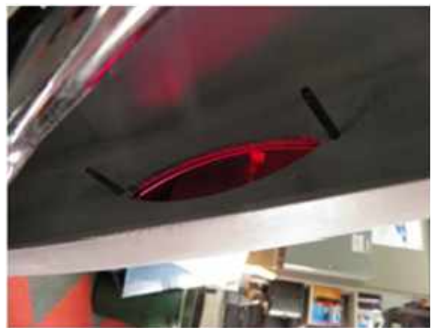
10. Slide the bezel with the set screws installed through the fender/bag and then slide the light box over the two studs and secure it with the two nuts provide.
