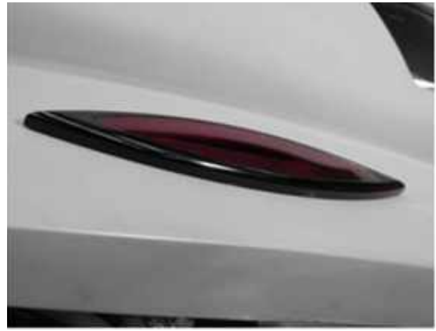
14. The bezel can flex slightly to adjust to the curved surface.
