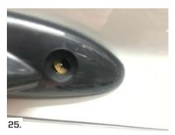
Be careful here NOT to cross thread the mount screw here! Here's a few tips to avoid cross threading these 2 screws:
