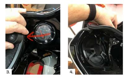
Next, using a plastic pry tool or a medium standard screw driver blade (TIP: wrap blade in masking tape to protect paint) pry up the inside upper corner of the speaker grill until it snaps free. (Fig #3 / #4) At the bottom outside corner of the speaker housings you'll find a #T-27 Torx head screw, remove it at this time. (Fig #5)
