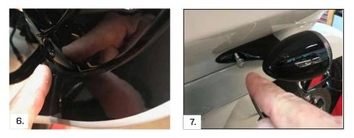
Continuing, locate the two #T-20 Torx head screws that hold your fairing wind guards on (locate on fairing outer edges below glove box doors) remove the lower screw only on each side (Fig #6). The last (2) screws to remove will be the 1/4x20 allen heads that bolt through the stock turn signal bodies on each side of the fairing. (Fig #7)
