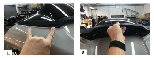
Removing your outer fairing per your factory service manual. First remove the (4) wind screen screws, two on the right and two on the left. (Fig #1)
