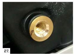
6B. You can also use a drift to insert in the treaded hole and gently pry the outer fairing hole and threaded bushing hole into alignment so you can get the screw started. Make sure the drift is deep in the bushing so as to not potentially damage threads near the outside of bushing where screw needs a clean "start"... Jack likes this method... (Fig #28)
