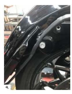
3. Slide rear fender into place with front of rear fender touching tire. Raise the back of rear fender upwards until mount lugs slide into their intended pockets. Install (2) Torx screws removed in Step 1 to hold fender in place. Finger tighten only at this time (Fig #3 | #4)
