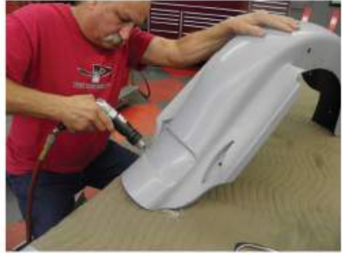
Drill pilot holes, then drill holes using a 7/32" bit.
