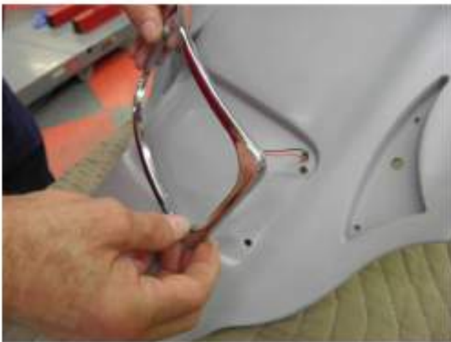
Mount frame. CAUTION: Do not torque set screws into frame. Lightly seat only.
