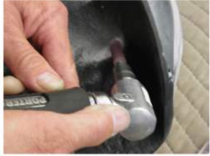
Flatten spots around holes on the underside of the fender to help the nuts sit flat.
