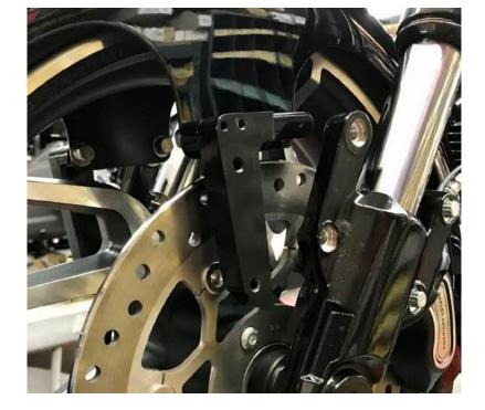
3. Slide fender in place over tire & repeat step #2 only this time with the bracket marked "L" on the left side (Fig # 4) Again, BLUE *LOCTITE*<sup>®</sup> and finger tighten only.
