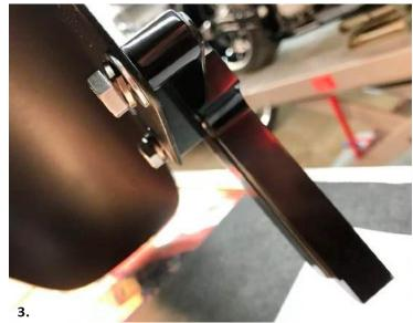
Note: Right & Left are determined The "R" faces outside surface of fender only when sitting on bike. Remember to, BLUE LOCTITE® and finger tighten at this time (Fig #3)
