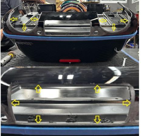
FEEL IF EDGE OF ROLL PAN AND THE EDGE OF TRUNK ALIGN NICELY. IF NOT, YOU *MAY* HAVE TO ENLARGE THE MOUNTING HOLES. OURS ENDED UP AT <sup>3</sup>/<sub>4</sub>" IN DIAMETER.
