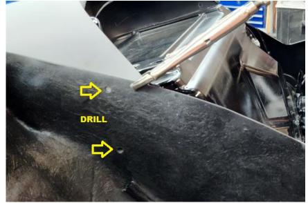
NOTE: THE UPPER-HOLE IS INTO TRUNK AND THE LOWER ONE THRU THE ROLL PAN.
