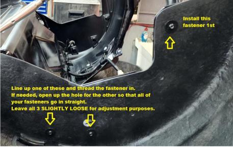
NOTE: Because mounting lugs glued in from the factory and can be a little off. Install top fastener 1<sup>st</sup>. (seems to be consistent) Then line up one of the 2 bottom holes and start that (leaving it slightly loose). Then open up the other hole so that it goes in straight. You may not have to
