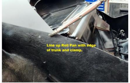
CHECK THAT THE CORNER OF THE ROLL PAN IS IN PLACE (ALONG THE EDGE OF THE TRUNK EDGE. THEN SNUG DOWN THE MOUNTING BOLTS. YOU ARE READY TO DRILL THE TWO REAR MOUNT HOLES 5/16" DIA.
