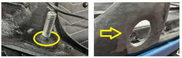
THE <sup>1</sup>/<sub>2</sub>" FLAT WASHERS ARE TO BE USED 1<sup>ST</sup> AT BASE OF THE STUD, THEN THE THICK WASHERS, THEN THE STRAP ACROSS THE PLATE FRAME BOX (STUD TO STUD). USE NON-LOCKING NUTS AT THIS TIME & SNUG DOWN, DO NOT OVER TIGHTEN!
