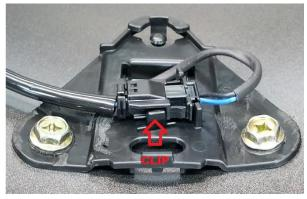
REMOVE THE TWO MOUNTING SCREWS FROM LIGHT FIXTURE PLATE.
