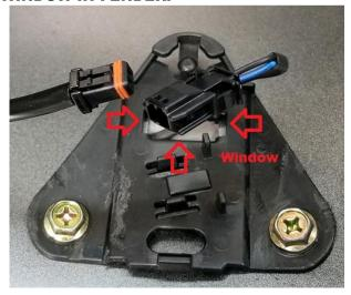
**PUSH CLIPS INTO FENDER + REMOVE COVER BASE FROM FENDER.**
